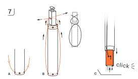
Tamper Evidence Seal: Thread the wire through holes at both ends of the capsule and into the plastic seal. Tighten the wires. Empress the plunger of the seal, until you hear a "click". You can press the unit face down on a hard surface. It is impossible to open the capsule without damaging the seal.
