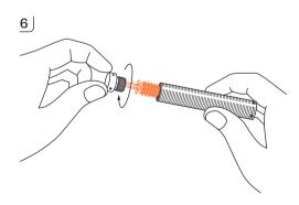
Upgrade module: Insert the core into the shell capsule and firmly screw on the cap.
