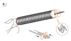
Once the complete password is assembled on the core, lock in the final cotter pin by pushing and pulling its pins. Check that both cotter pins are securely locked.
