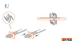
Insert a cotter pin into one of the core slots. Pull firmly in both directions to bend its pins to lock in place.
